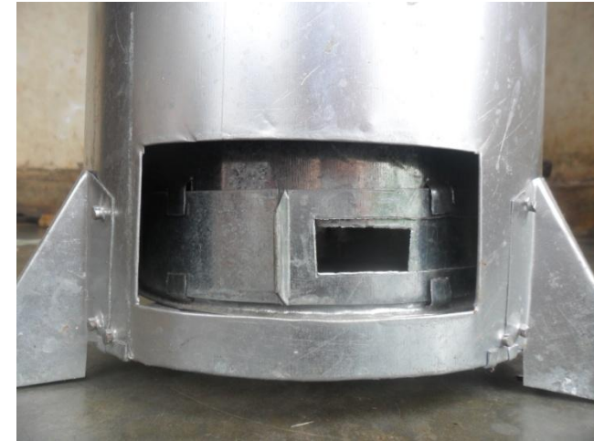
Picture 25: Primary air controller
