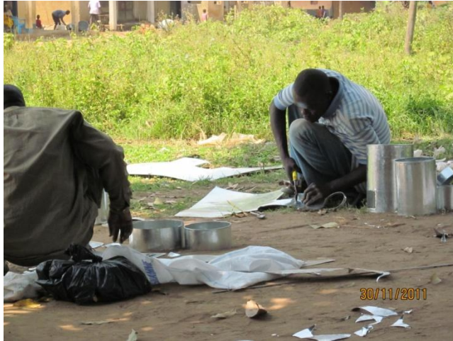
Picture 52: Cutting metal strips for the riser / pot stand combination
