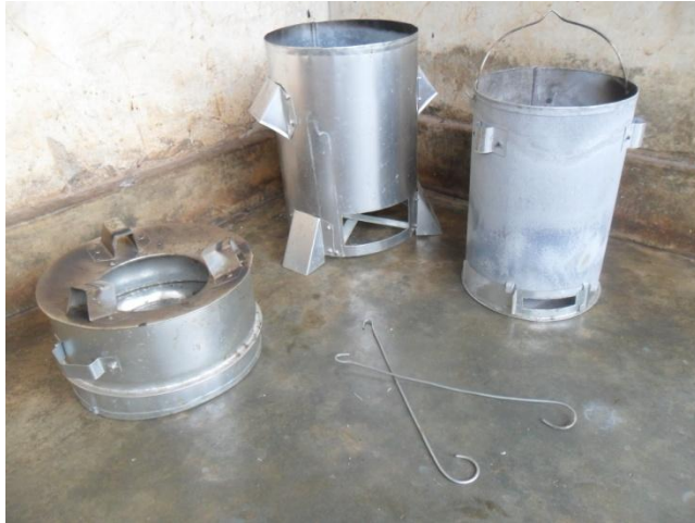
Picture 27: Four main components of the MWOTO stove
