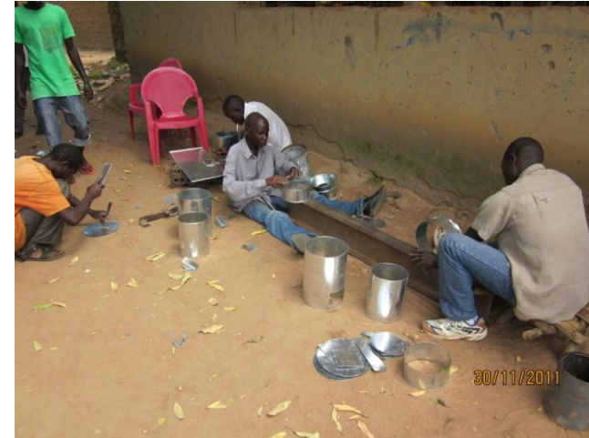
Picture 54: Manufacturing the concentrator disc ...
