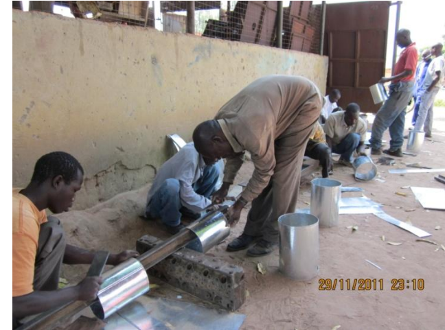
Picture 50: Producing cylinders
