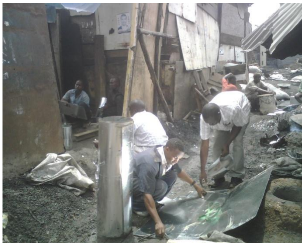
Picture 43: Taking measurements for the outer cylinder
