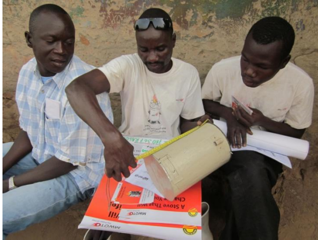
Picture 66: Measurement of stove dimensions
