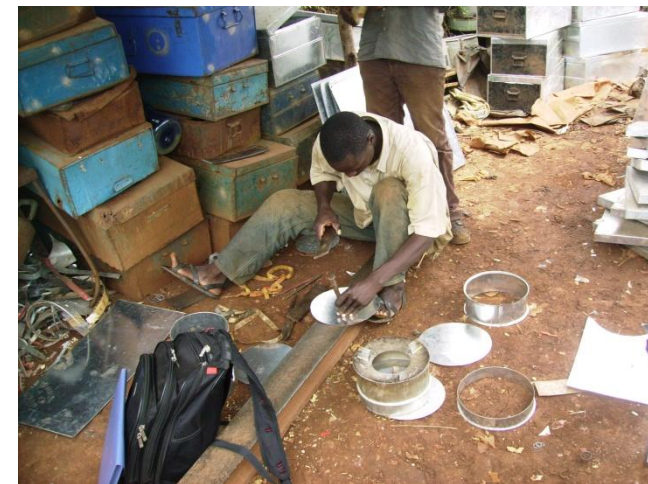
Picture 36: Construction of the riser / pot stand combination
