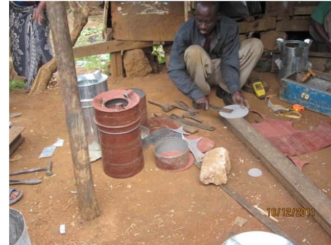
Picture 58: Producing a TLUD from scrap metal
